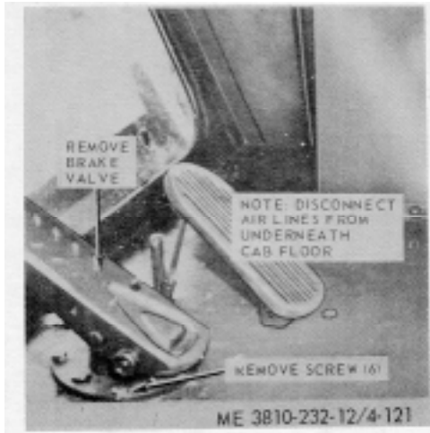
Figure 4-121. Brake valve, removal and installation
